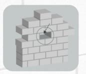
Use power tools to create grooves in the AAC blocks to accommodate electrical wiring and pipes.
