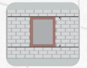
A coping beam should be constructed every 4 rows, and a 6/8 mm lintel should be placed above the windows.
