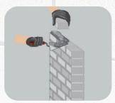
Arrange the blocks in rows on the prepared bed and continue building the wall until construction is complete.
