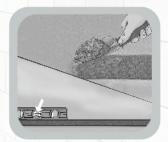
Using a sand-cement mix, lay the AAC blocks with the 'O' level side on the ground and ensure that the ridge grooves are leveled into the ground.
