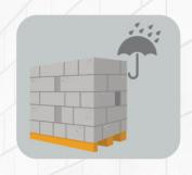
Ensure that AAC blocks are stacked on a flat and level surface and make sure to use blocks that are completely dry.
